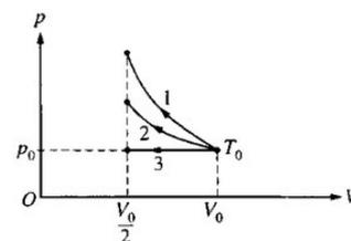
A certain quantity of an ideal gas initially at temperature  $T_0$ , pressure  $p_0$ , and volume  $V_0$  is compressed to one-half its initial volume. As shown above, the process may be adiabatic (process 1), isothermal (process 2), or isobaric (process 3).
