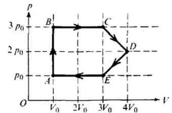
An ideal gas undergoes a cyclic process as shown on the graph above of pressure  $p$  versus volume  $V$ .
